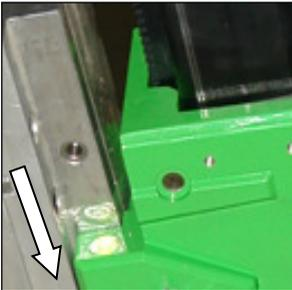
Insert the core drill with the attached mounting plate into the drill rig and lock it with the turnstile .
