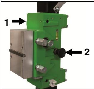
To unlock the carriage (1) pull out the lock knob (2).
