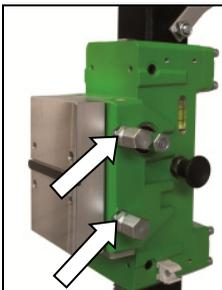
Move the machine holder upwards until it locks in the top position.
