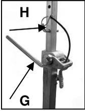
Position the drill rig. Position the quick action bracing unit as close as possible behind the support on the base of the rig or on the clamping head of the column. Fix the drill rig by turning the crank (G) clockwise. Secure in position by means of the appropriate bolt (H).
